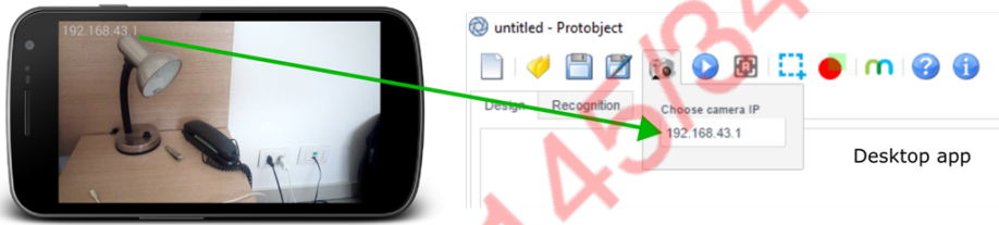
Fig. 1. A smartphone turned into a Wi-Fi camera that displays the IP address to connect.
